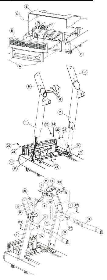
Position the right end of the ERGO FRONT CROSSBAR (#4) near the large access hole on the inside of the RIGHT UPRIGHT HANDLEBAR BRACKET (L).
